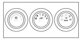
With this system you can control the heating, cooling, and ventilation of your vehicle. In-between modes are available by moving the right control knob between modes with symbols. The in-between mode will be a combination of the two modes that the control is selected between.
